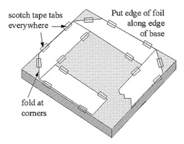
Cut a 6" wide piece of aluminum foil. Lay it on the base, withits edge along the edge of the base. Make a 6 1/2" gap in the corner where the foil begins. Then fold the foil over itself as shown above.
