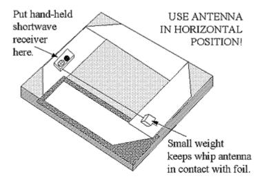
Put the receiver on the foil as shown, don't worry about electrical connection. Pull the whip antenna out, use a small weight to make sure the whip contacts the foil.
