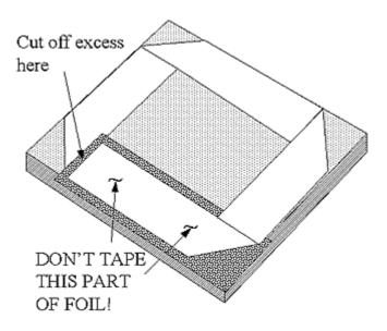
Leave the fifth flap of foil loose, cut off excess foil.
